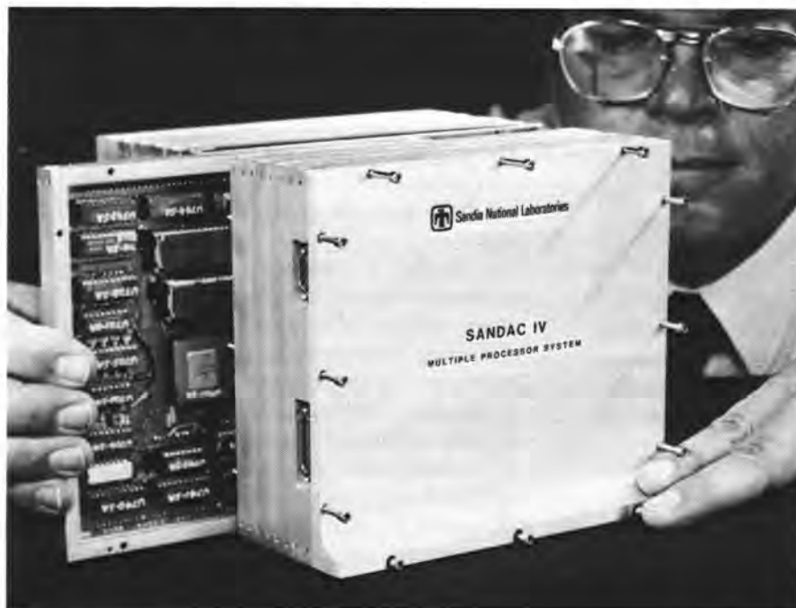
SANDAC IV can fit inside a weapon but has the computational power of a desk-sized computer. The SANDAC embedded computer series (V is an even more powerful version) may someday lead to truly "smart" weapons.
